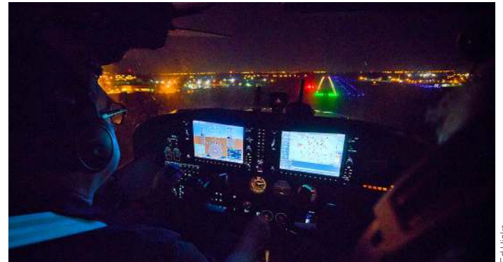
Above Why is 'red-green' an issue for pilots? You wouldn't want to get the PAPIs and runway lights mixed up in the above view, would you?
